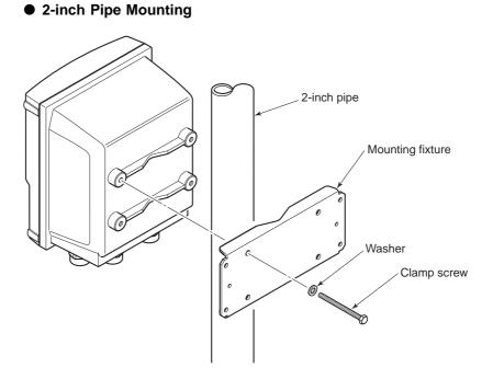
Pass the four clamp screws through the mounting fixture, position it on the 2-inch pipe, and then fasten the AXFA11 in place.
